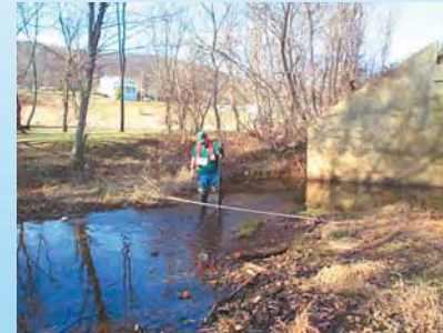
Stream Gaging with Current Meter (Shallow rivers)
