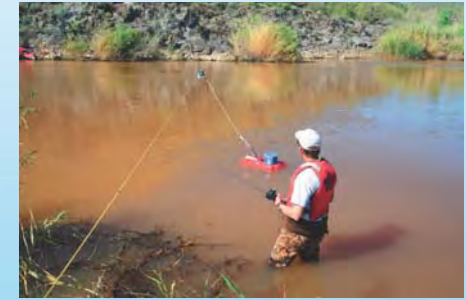
Stream Gaging with Acoustic Doppler Current Profiler (Shallow rivers)
