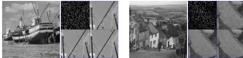
Figure 2: Comparison of interpolation results, considering BP and dHBP on the 512 \times 512 Boat and Hill images, with 80% of their pixels missing uniformly at random. The left-most and third images show the dHBP reconstructions of Boat and Hill, respectively. The second and fourth images show two enlarged regions as in Figure 1.
