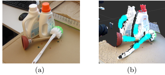
Fig. 1. (a) An RGB image of a typical scene. (b) Handle-like grasp affordances localized using our algorithm highlighted in cyan.
