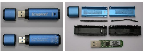
Fig. 29. DataTraveler Vault Privacy 3.0 before and after opening plastic case
