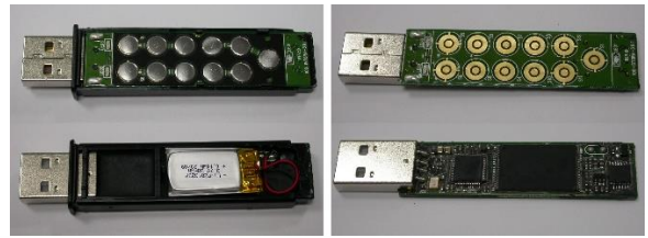
Fig. 47. Datashur before and after epoxy removal
