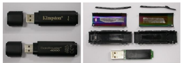
Fig. 34. DataTraveler DT4000 before and after opening its plastic case
