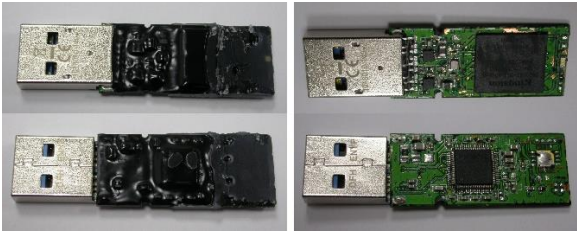
Fig. 51. Integral Crypto before and after epoxy removal
