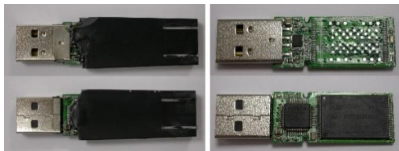
Fig. 3. IronKey device before and after epoxy removal
