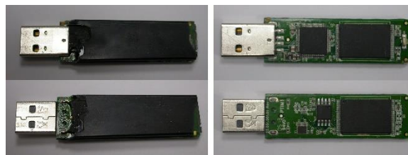
Fig. 2. IronKey device before and after epoxy removal
