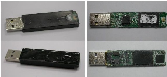
Fig. 5. IronKey D2 before and after epoxy removal
