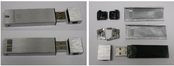
Fig. 11. IronKey S200 before and after opening its metal case
