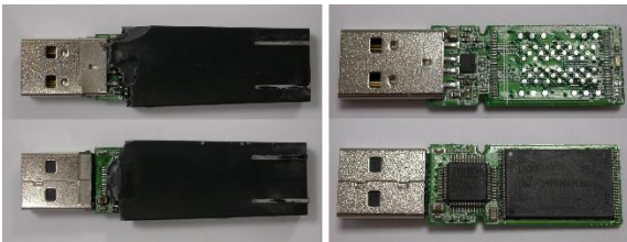
Fig. 20. IronKey D80 before and after epoxy removal
