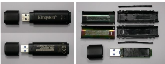
Fig. 27. DataTraveler DT4000G2 before and after opening its plastic case
