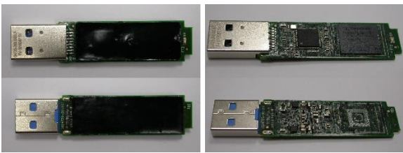
Fig. 28. DataTraveler DT4000G2 before and after epoxy removal
