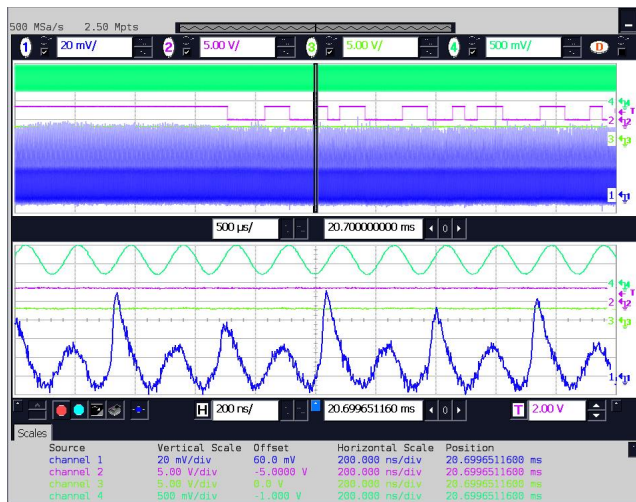
Fig. 9 Frequency locking at 5.720 MHz (phase shift -50^\circ )
