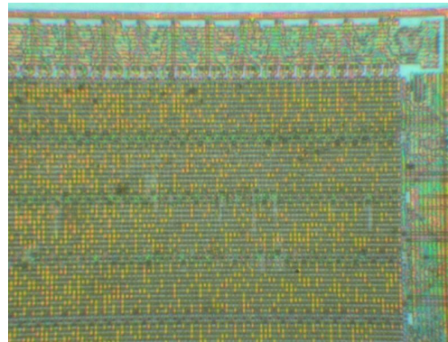
NEC \mu PD78F9116 microcontroller 0.35 \mu m
