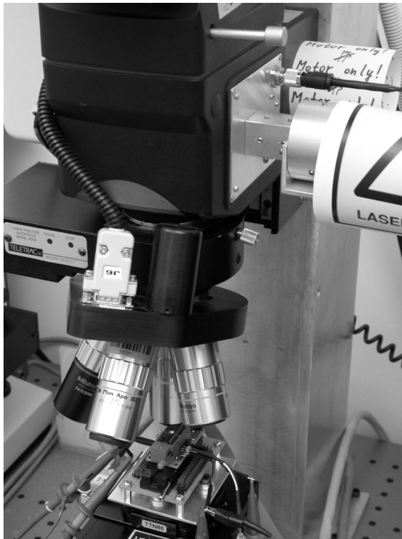
Fig. 2. Test setup for semi-invasive analysis
