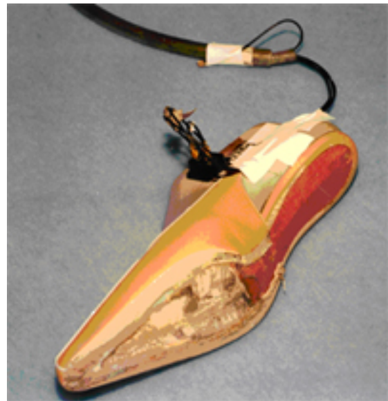
Figure 4 Attaching the acceleration transducer to the last
