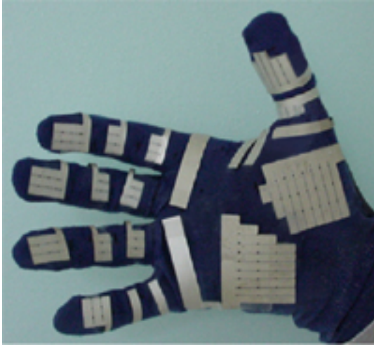
Figure 3 Mechanical lay-out of the new prototype. Distribution of the sensors on the hand
