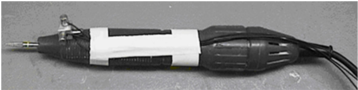
Figure 7 Attachment of the acceleration transducers to a straight grinder
