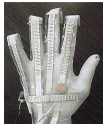
Figure 2 First prototype comprising 51 sensors
