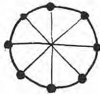
Marks for Post Holes
