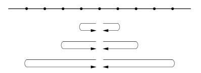
Figure 3: Paths of messages of process P<sub>i</sub> in algorithm HS.
