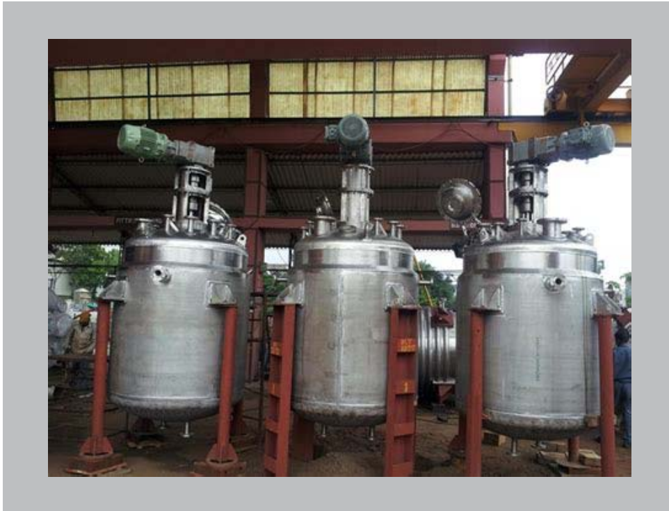
Figure D-2. Chemical Reactor Vessel
