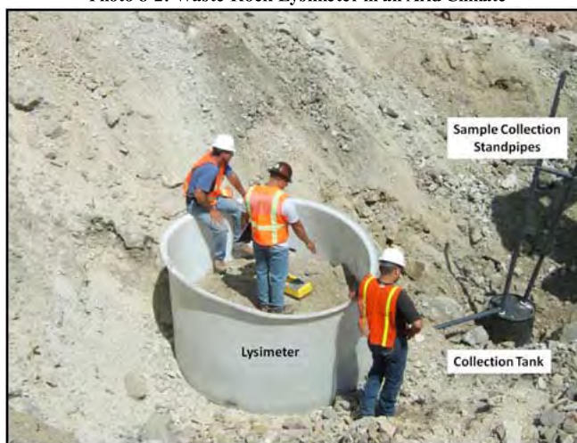
Photo 8-2: Waste Rock Lysimeter in an Arid Climate
