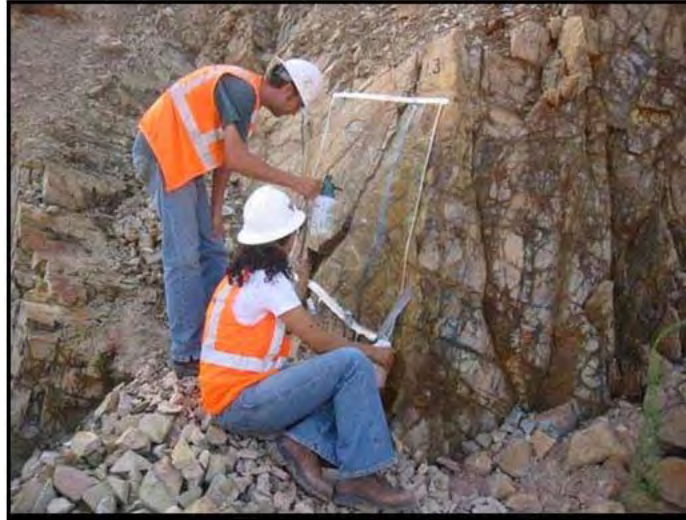
Photo 8-1: Collection of a Wall Washing Sample from a Pit Face
