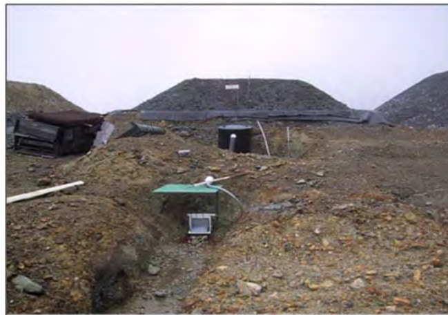
Figure 5-13: Test Cells for Waste Rock – Grasberg Mine, Indonesia
