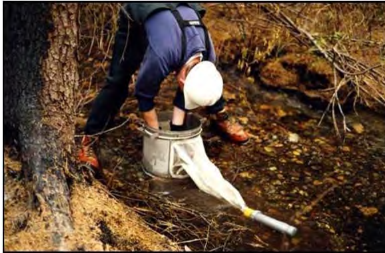
Photo 8-5: Benthic Macroinvertebrate Sampling with a Hess Sampler
