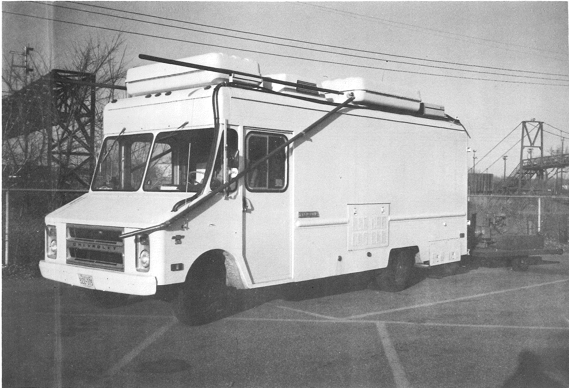
Figure A1. University of Minnesota Mobile Laboratory (UMML) as configured for the Los Angeles Roadway Study in 1976. Note upper and lower sampling intakes and towed generator.
