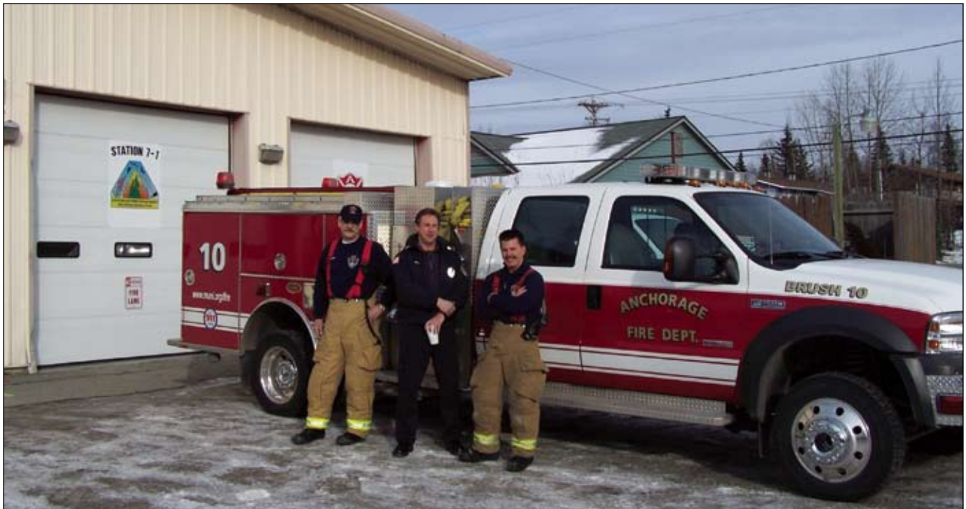
Brush 10, a KME Mini Pumper, is a wildland engine equipped with compressed air foam. It operates as a fully functional structural firefighting engine with the capacity to travel over challenging roads. It is housed at Station 10, Rabbit Creek.
