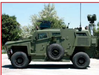
Xstream – A 16 Ton all terrain 4X4 MRAP, up to 7 people, KE Stanag 2 and Mine protection Stanag 3a+2b
