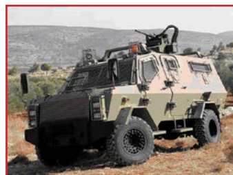
Wolf – A 9 Ton multi purpose 4X4 APC, up to 8 people, KE Stanag 2 and Mine protection up to Stanag 1
