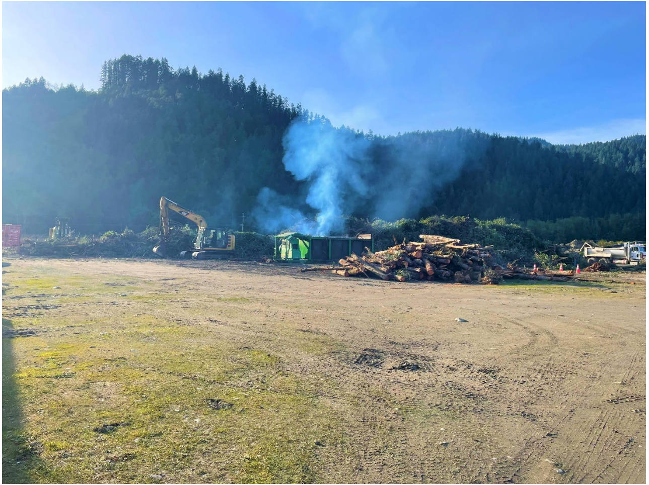
Image 10 Air Curtain Burner being utilized for storm damage clean-up in Willow Creek.
