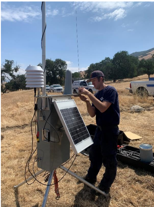
Portable RAWS installation in preparation for a prescribed fire in Battalion 1
