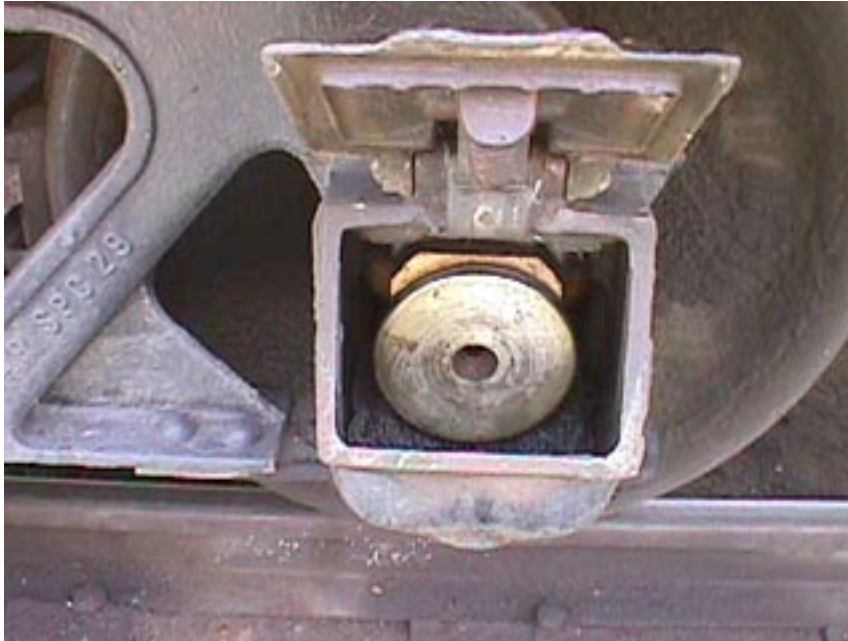
Photograph 3-6. Old Style Wheel Bearing (Journal Box Type)
