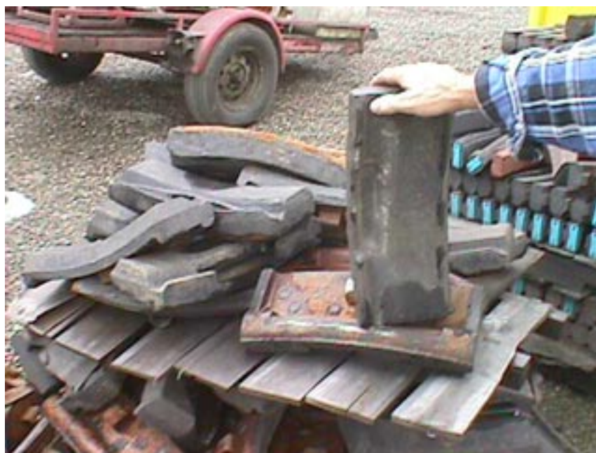
Photograph 6-3. Switch Engine, Flanged Cast Shoes (has more braking power)
