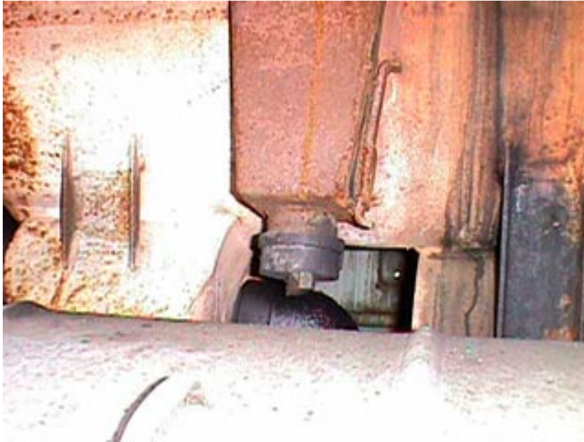
Photograph 5-9. Cup-Type Carbon Trap (Note Locking Mechanism on Right Side)
