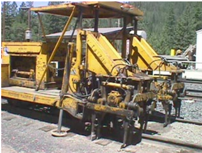
Photograph 7-8. Tie Replacement Equipment
