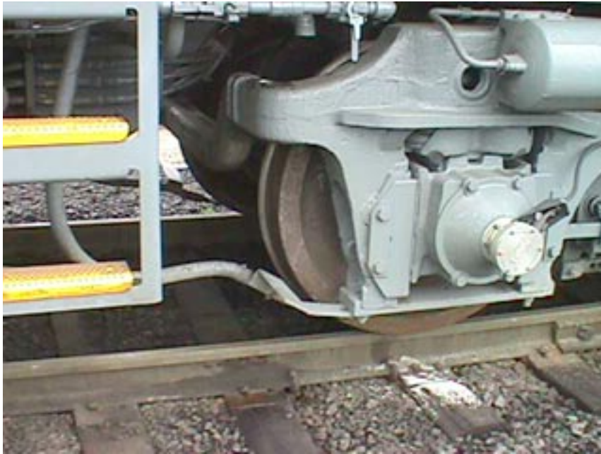
Photograph 3-3. Sand Dispenser for Traction
