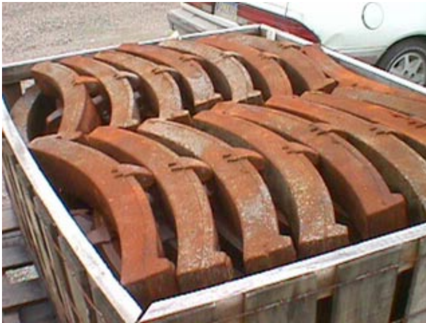
Photograph 6-1. Switch Engine, Cast Brake Shoes with Wear Indicators
