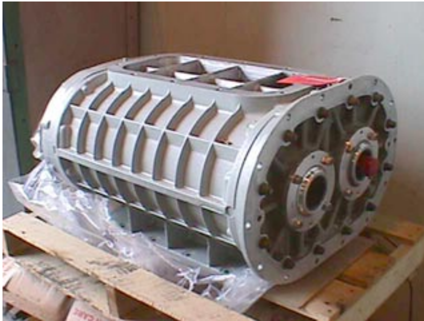
Photograph 5-2. Roots Blower - EMD
