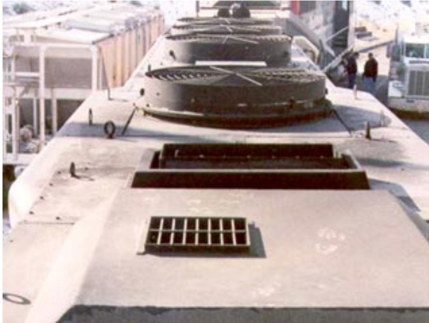
Photograph 5-15. Top of Locomotive, Exhaust Stack
