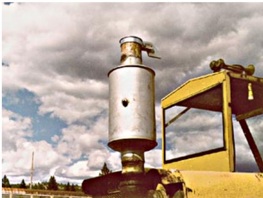
Photograph 5-7. Retention Spark Arrester with Plug
