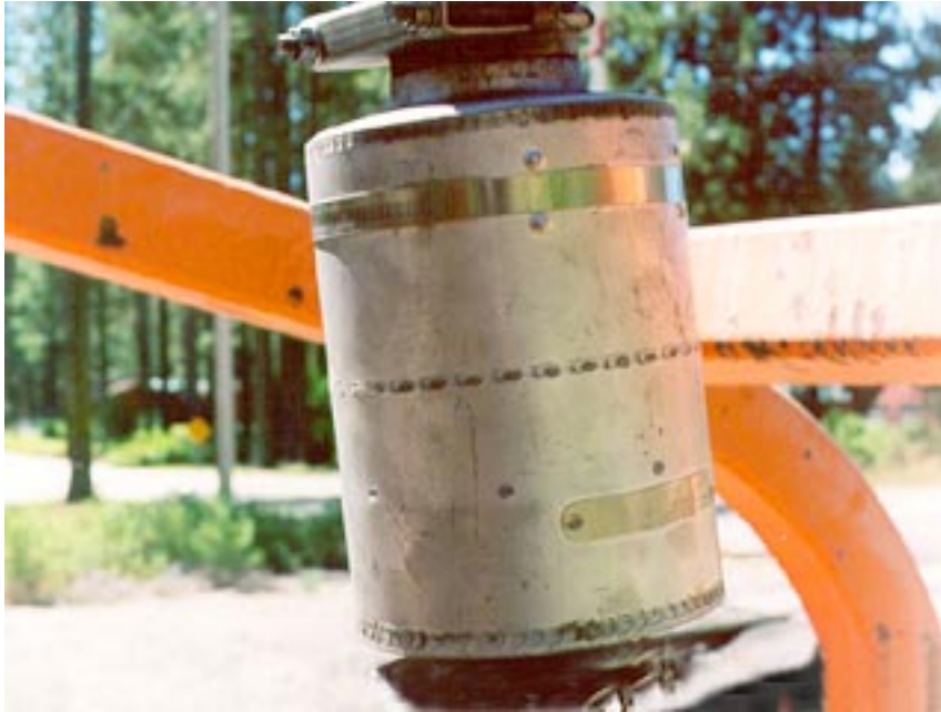
Photograph 10-1. Spark Arrester on Bulldozer
