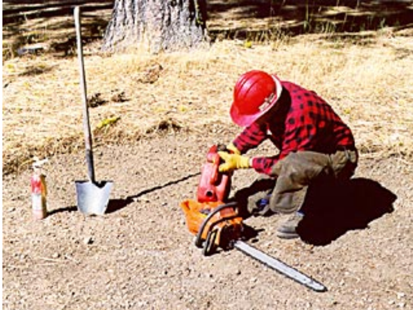
Photograph 5-3. Chain Saw Being Refueled
