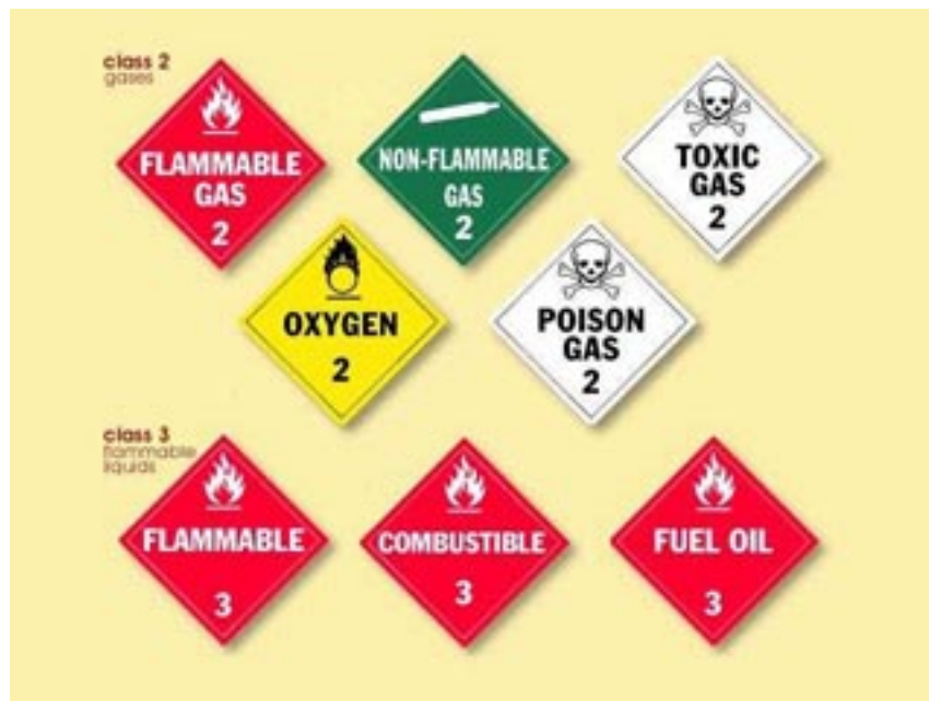
Figure 12-1. Common Hazardous Materials Placards
