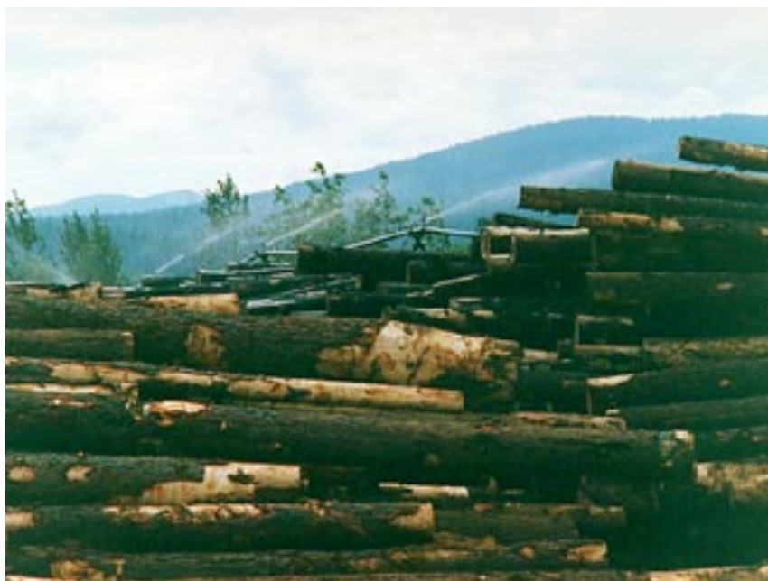
Photograph 13-4. Sprinklered Log Deck
