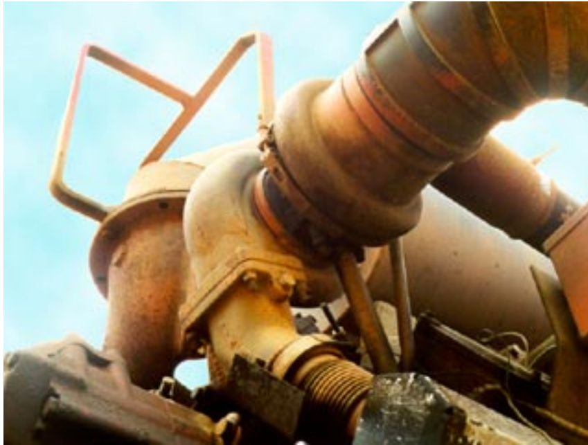
Photograph 9-5. Turbocharger on Equipment
