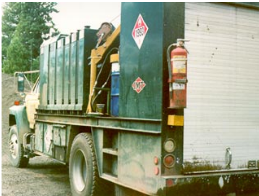
Photograph 5-5. Large Fire Extinguisher on Mechanic's Truck
