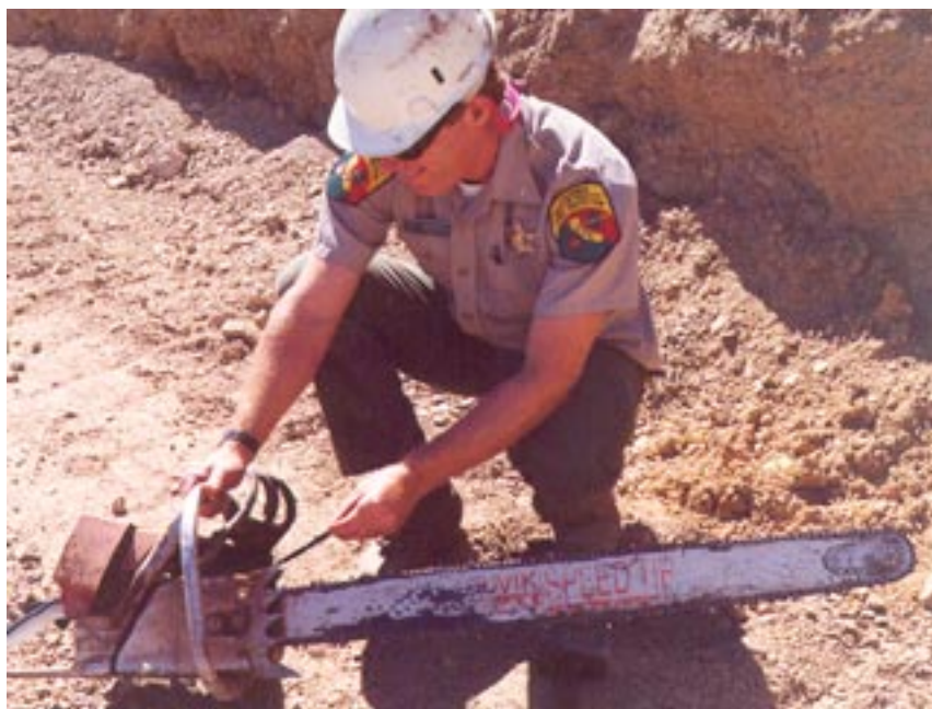
Photograph 9-3. Chain Saw With Properly Attached Bumper Spike and Heat Shield
