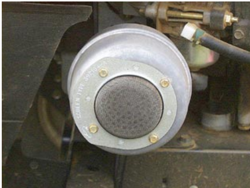
Photograph 4-8. Attrition Spark Arrester (Screen Type)
