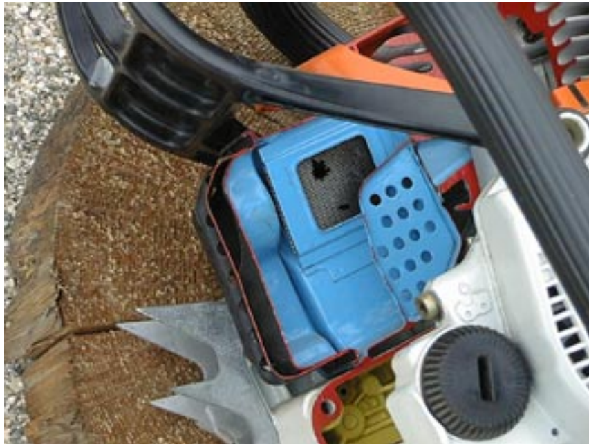
Photograph 9-2. Burned Out Chainsaw Spark Arrester Screen
