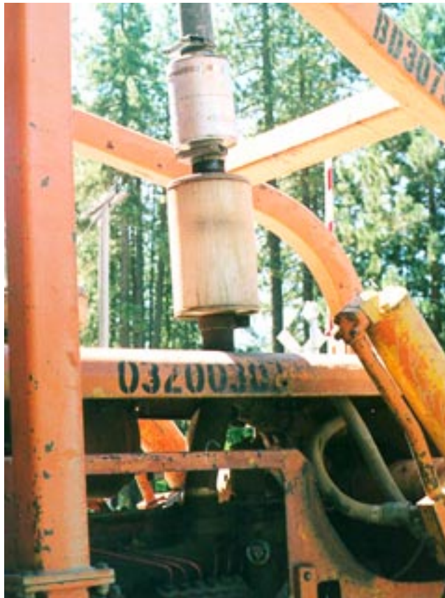
Photograph 9-7. Machine Equipped with Both a Muffler and Spark Arrester
