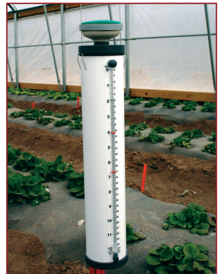
Figure 13: Atmometers are popular for measuring soil moisture levels. They offer a simple way to measure on-site evapotranspiration.
