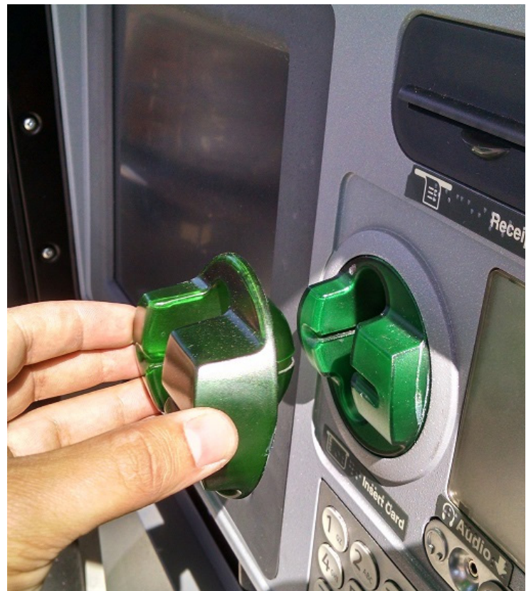
A skimmer being installed on an ATM.
