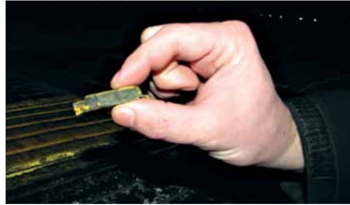
Regular power washing stretches the interval between repainting and reduces the associated risk for "homegrown FOD" from excessive paint buildup.
