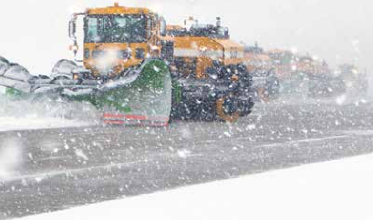
A new fleet of MB5 plow/broom vehicles helps IND clear runways faster.
