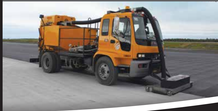
AMV Recover glycol, remove and manage runway rubber, strip and collect falling paint with the Triverus AMV.
