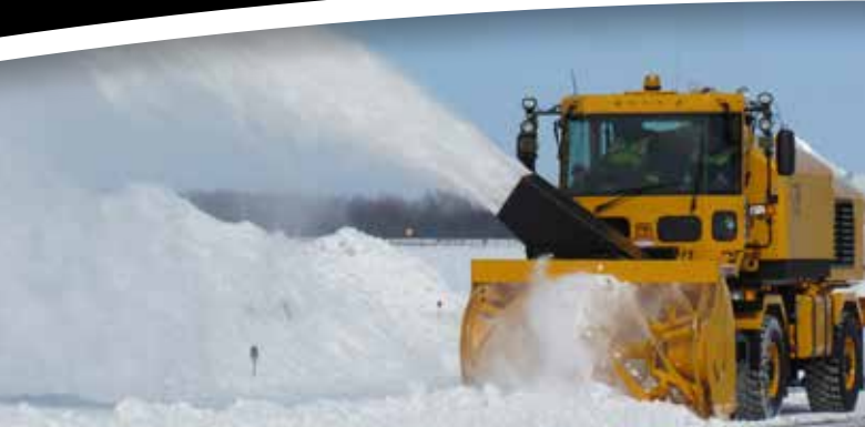
MB4 The MB4 snow blower's standard 1175 horsepower clears airports at up to 7500 tons per hour.
