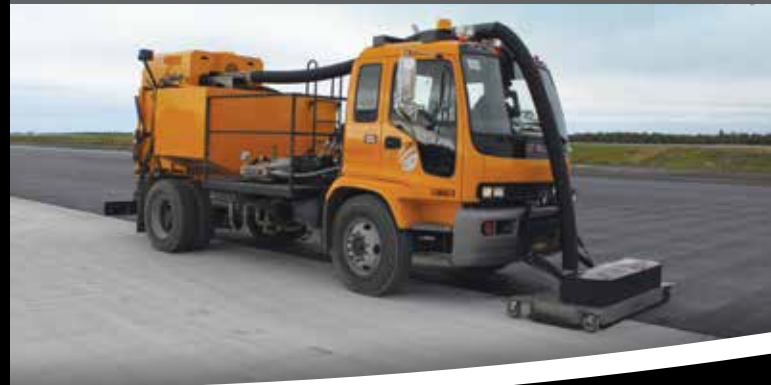
AMV Recover glycol, remove and manage runway rubber, strip and collect falling paint with the Triverus AMV.
