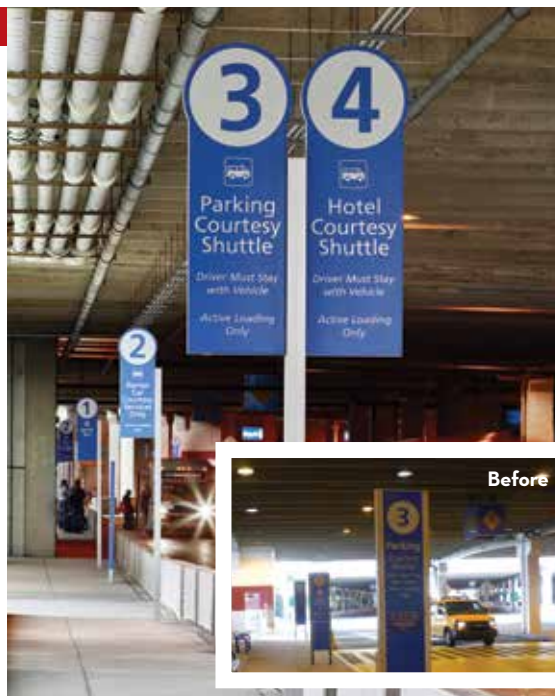
New freestanding signs along curbs near baggage claim areas identify zone assignments for various ground transportation services. A single-post design and ample clearance allow pedestrians to walk underneath. Previous double-post signs blocked more of the sidewalk.
