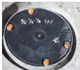
Active sensors, above, are a crucial component of the airport's new ice warning system from ASFT.
