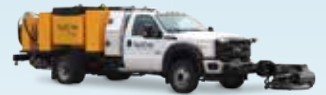
The CY4006ST – Rubber and paint removal with the power of a Cyclone on a compact and affordable platform. Ideal for contractors and low volume airports.
