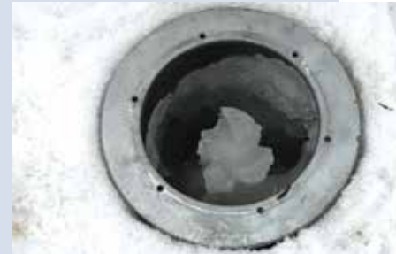
Left: An evacuation wand clears ice, melting water and other extra materials from the can. Right: Close-up of partially completed clearing process.
