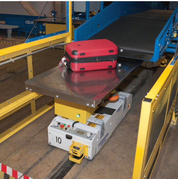
Automated carts transport flagged bags from the conveyor system (left), to screening inspectors, and back again (right) to eliminate lifting and carrying.
