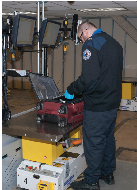
Automated carts transport flagged bags from the conveyor system (left), to screening inspectors, and back again (right) to eliminate lifting and carrying.
