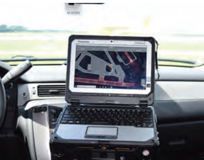
38 BWI Marshall Uses Vehicle Tracking System to Improve Airfield Management
