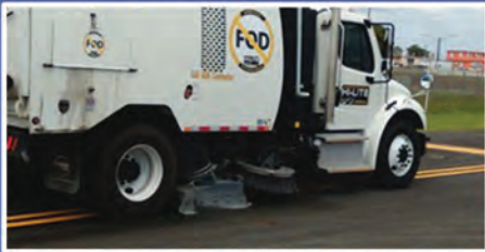
VACUUM AND BRUSH REMOVAL OF DEBRIS
