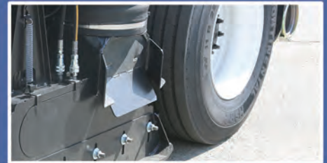
HIGH VELOCITY BLAST AIR TO PUSH MATERIAL OFF SURFACE
