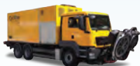
The CY4006HT – Heavy-duty Cyclone Technology cleaning power on a Heavy-duty truck. High water capacity allows for over 5 hours of operating time.
