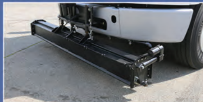
POWERFUL MAGNET TO COLLECT FERROUS MATERIAL
