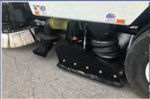
VACUUM AND BRUSH REMOVAL OF DEBRIS
