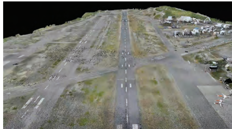
The drones captured images and data for a runway markings assessment and other airfield surveys.
