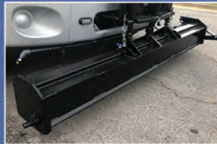
POWERFUL MAGNET TO COLLECT FERROUS MATERIAL
