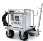
ITW GSE 1400 28 VDC GPU
