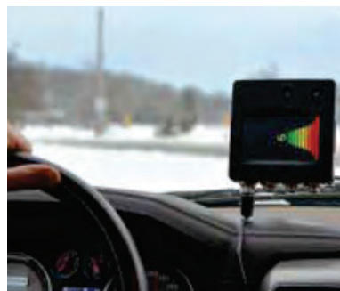
R'Over™ System In-Cab Visual/Audible Display
