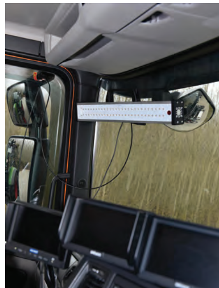
CleanRide UV-C uses ultraviolet-C light to disinfect vehicle cabs.
