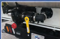
GLYCOL RECOVERY FOR PICKING UP DE-ICING FLUID
