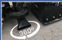
HIGH VELOCITY BLAST AIR TO PUSH MATERIAL OFF SURFACE
