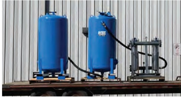
The airport has spent about $2 million on the PFAS issue, including point-of-entry water treatment systems (shown left) for some nearby homes and a remediation system (shown right).
