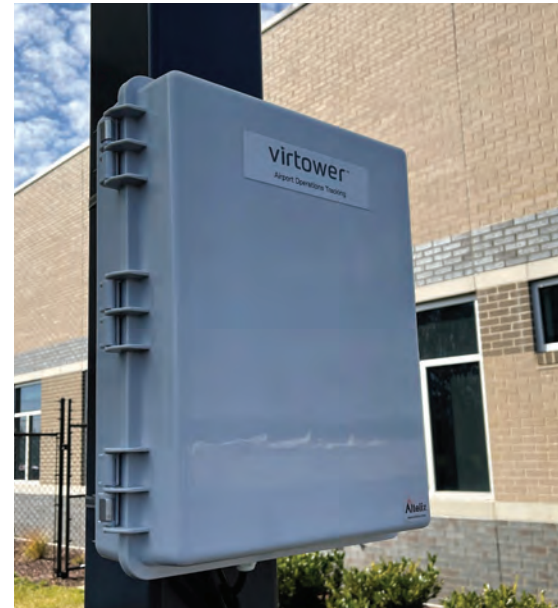
The sensor box was installed on a light pole adjacent to the terminal.
