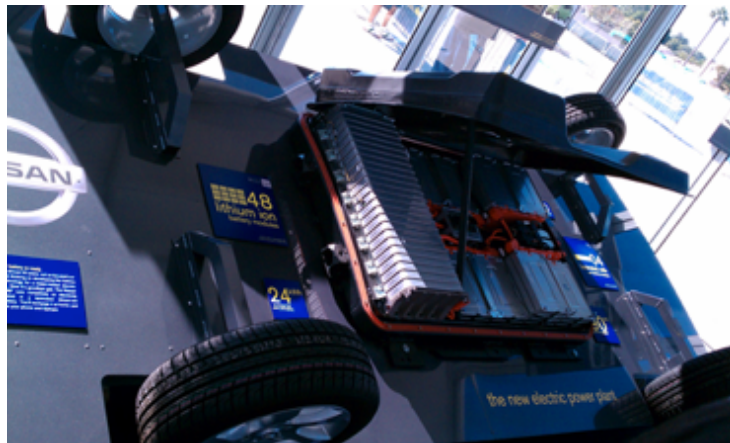
Nissan Leaf battery power plant
