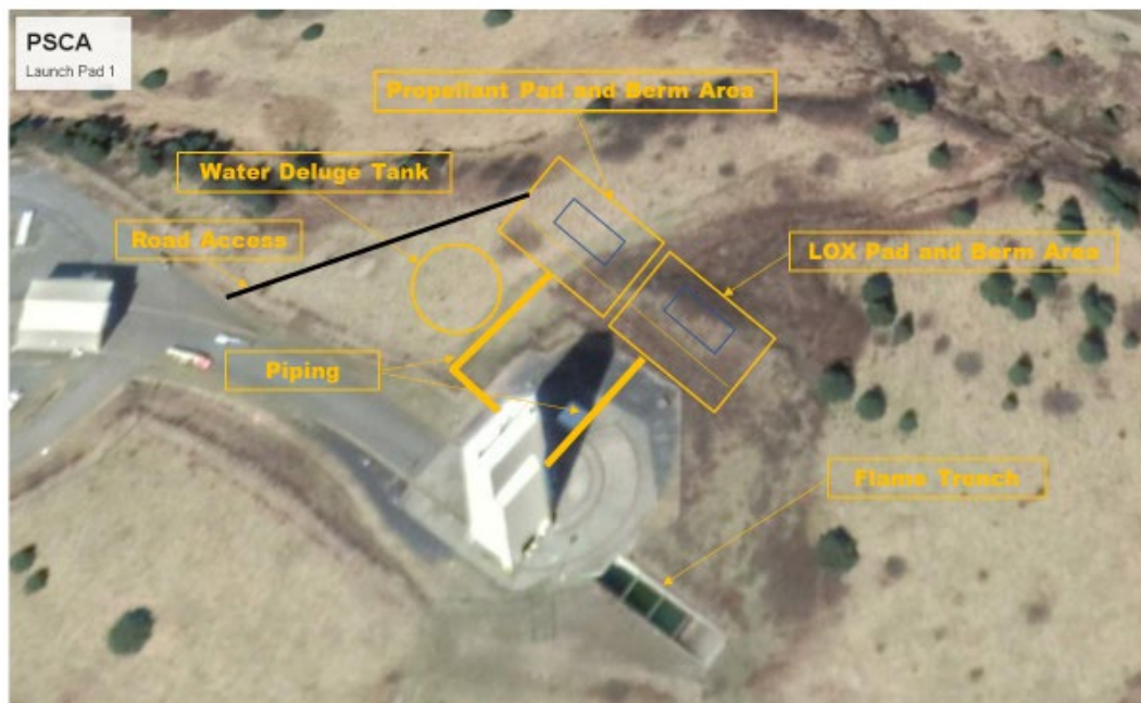
Figure 5-3: Launch Pad 1 Development Alternative
