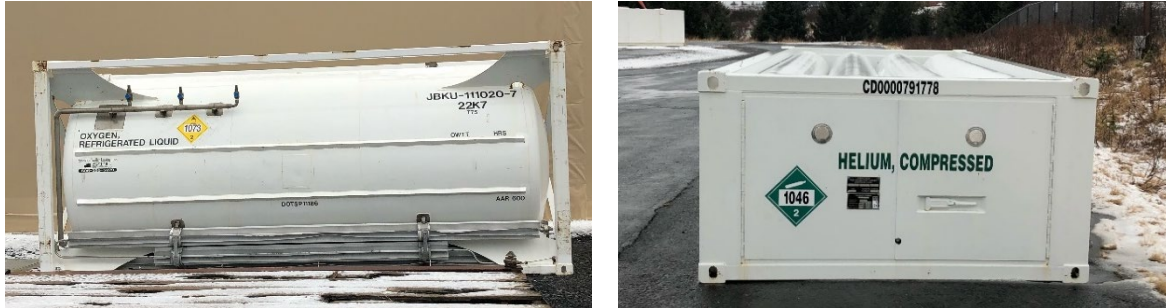
Figure 2-12. Bulk LOX and Helium Storage
