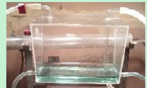
Photocatalytic Reactor for Hydrogen Recovery
