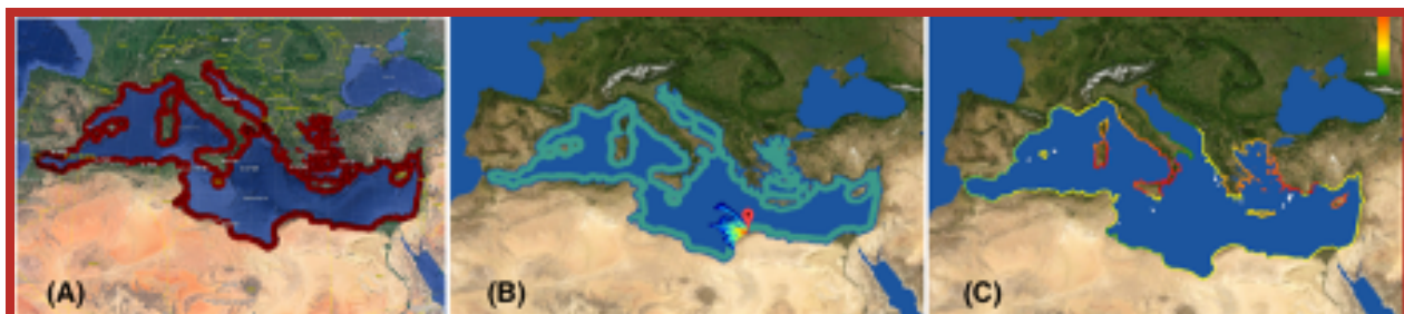
Figure 3. (A) in red, the sampling release points; (B) in light green, the sampling belt (10 to 50 km from the coast, 10 km sampling rate) together with a mean trajectory of the spill (red pin-point); (C) hazard mapping of the Med. Sea: different colors denote the different hazard levels for each coast segment.
