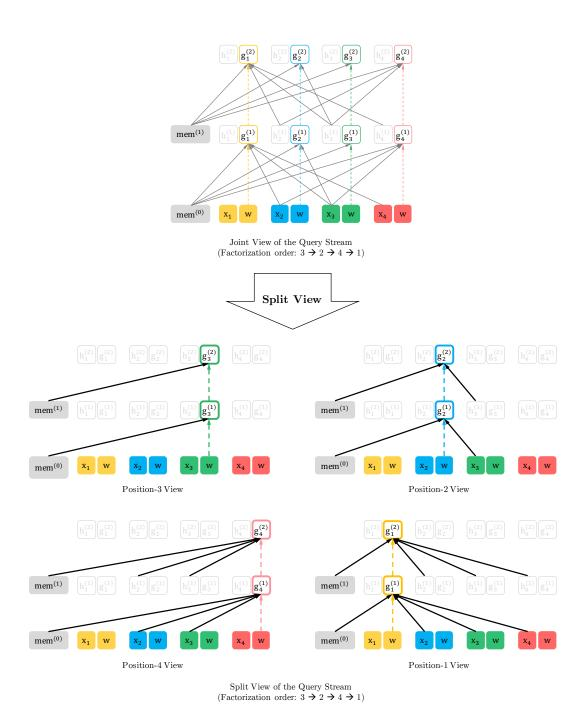
Figure 6: A detailed illustration of the **query stream** of the proposed objective with both the joint view and split views based on a length-4 sequence under the factorization order [3, 2, 4, 1]. The dash arrows indicate that the query stream cannot access the token (content) at the same position, but only the location information.
