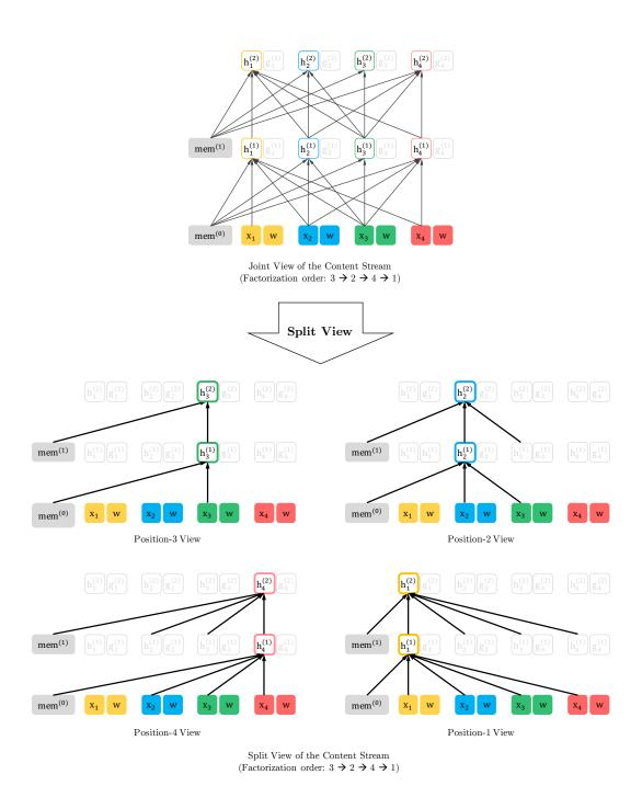
Figure 5: A detailed illustration of the **content stream** of the proposed objective with both the joint view and split views based on a length-4 sequence under the factorization order [3, 2, 4, 1]. Note that if we ignore the query representation, the computation in this figure is simply the standard self-attention, though with a particular attention mask.
