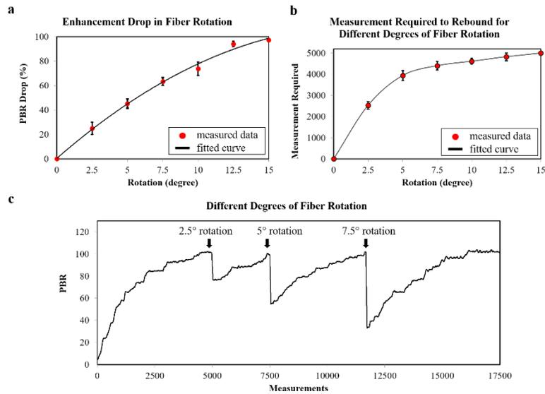
Fig. 6 a) Relationship between fiber rotation and PBR drop. b) Measurement required to rebound for different degrees of fiber rotation. Each dot in a) and b) is averaged from 5 executions and the error bars show the standard deviation of the measurements. Optimizations in a) and b) are realized by the DMA. c) Experimental focusing performance of the DMA in response to  $2.5^\circ$ ,  $5^\circ$ , and  $7.5^\circ$  fiber rotation.
