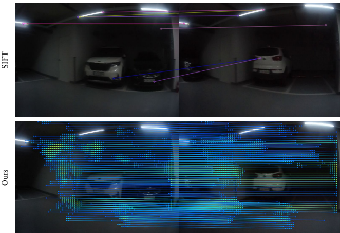
Fig. 3. Failure cases of the sparse matching methods. Sparse matching methods rely on interest points that have distinctive appearances. They tend to suffer from textureless walls in indoor parking lots.
