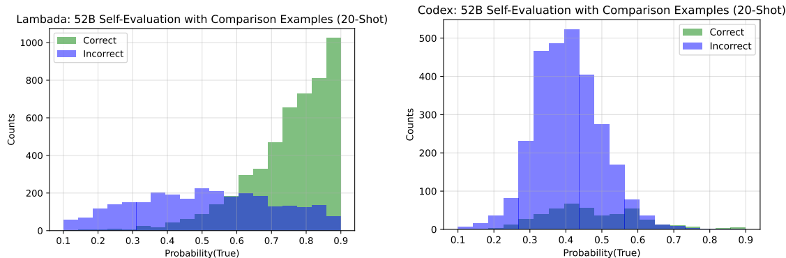
Figure 10 Models self-evaluate their own samples by producing a probability P(\text{True}) that the samples are in fact correct. Here we show histograms of P(\text{True}) for the correct and incorrect samples, in the evaluation paradigm where models also see five T = 1 samples for the same question, in order to improve their judgment. Here we show results only for Lambda and Codex, as these are fairly representative of short-answer and long-answer behavior; for full results see Figure 28 in the appendix.
