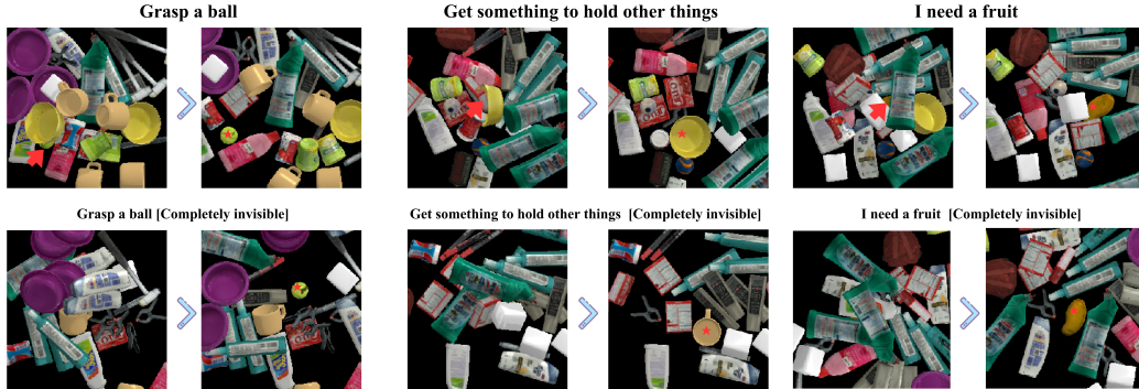
Figure 4: Heavy Clutter cases in simulation. The target objects are labeled with stars.
