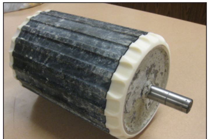
Canton High School students designed and created a tapered end for a roller used on a powered cement screed as part of a PLTW course. (Photos courtesy of Canton School District)
