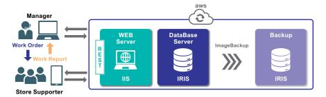
PIT has standardized on a REST API for screen-based processing to and from PCs and smartphones.
