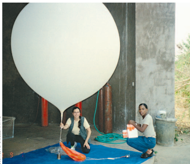
Anne Thompson NASA scientist, and Agnes Phahlane, a meteorologist of the South African Weather Service, prepare for a balloon launch during the SAFARI-2000 campaign in Zambia. The balloon carried both an ozonesonde instrument to measure ozone and a radiosonde to measure temperature, pressure, and relative humidity—conditions that can affect ozone concentrations and distribution.
