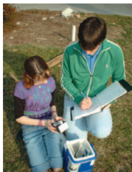
Gianna D'Emilio and Chris Hanawalt take aerosol measurements using a handheld sun photometer.
